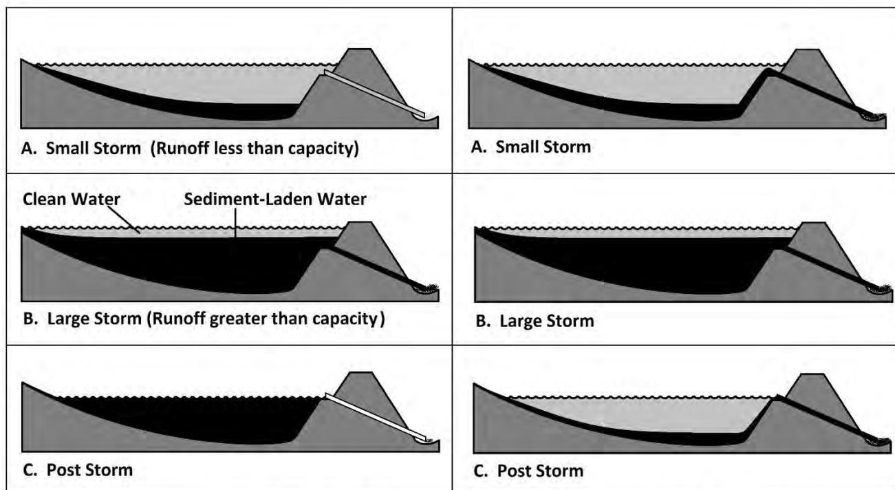
**Figure 1. Cross-sectional view of a pond with a surface-withdrawal spillway.**
